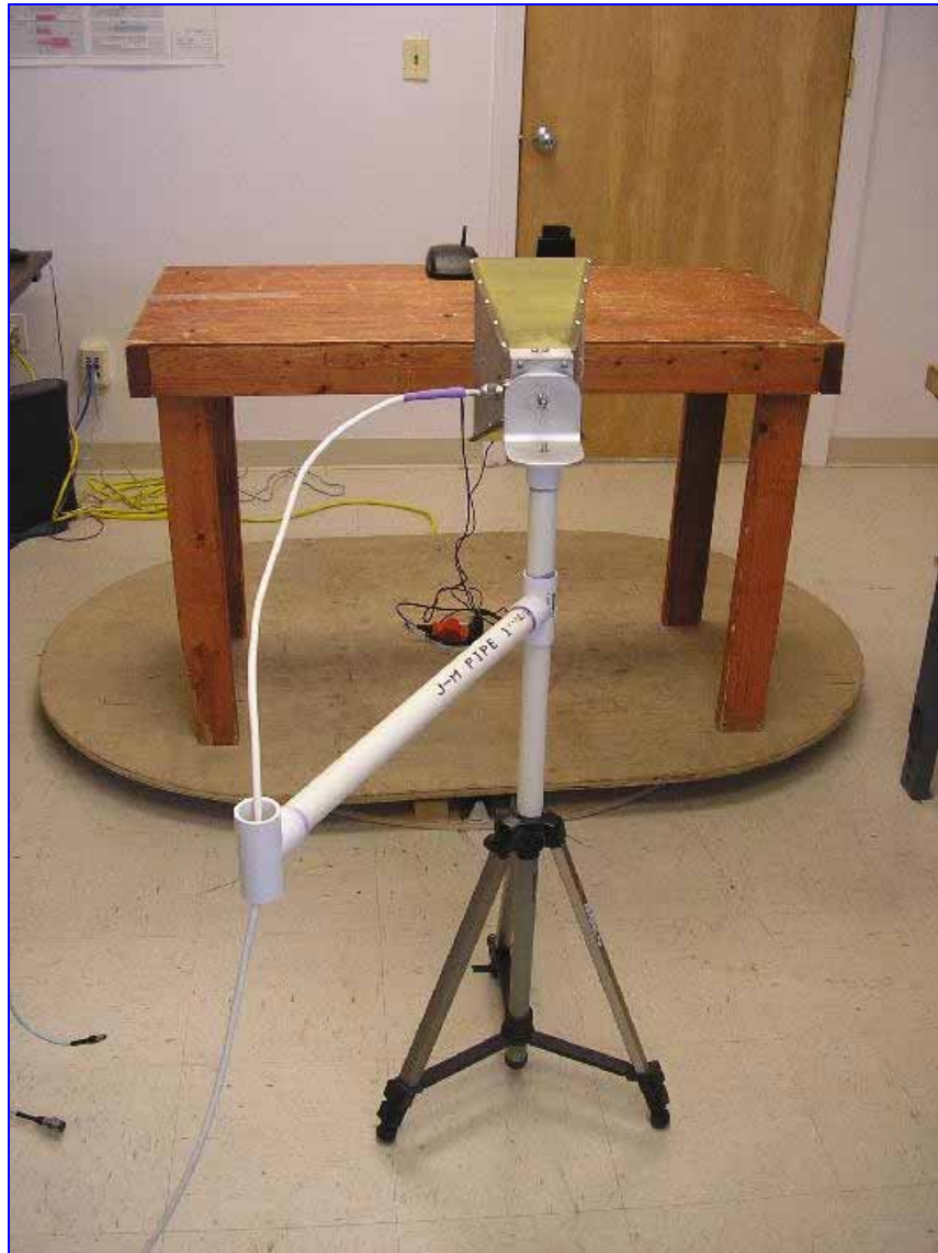
Photograph 2. Intentional and Spurious Emission Limits Test Setup
