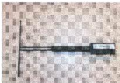
Figure 1 – Satimo COMOSAR Validation Dipole
