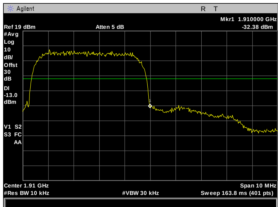
Plot 102. Band Edge Emissions, WCDMA, 1900 MHz Band, High Channel
