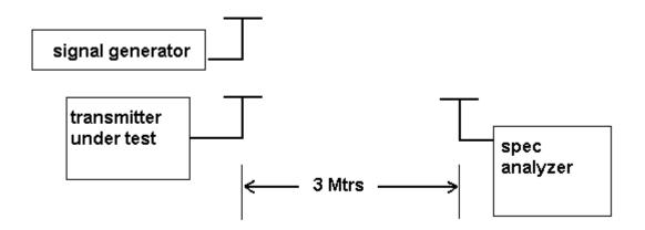
Equipment placed 80cm above ground on a rotatable platform.
