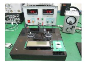
1. Connect Power supply(7.2V) to the JIG. Also connect WATT meter to JIG. Watt meter setting is 300mW.
