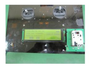
**2**.Insert Spectra Pro to the JIG. Turn ON the power of the JIG.
