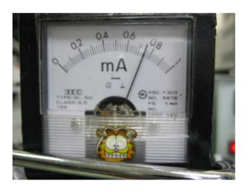
4. Check for the RF status (bounding fail). Readjust RFT coil again when encounter this problem.
