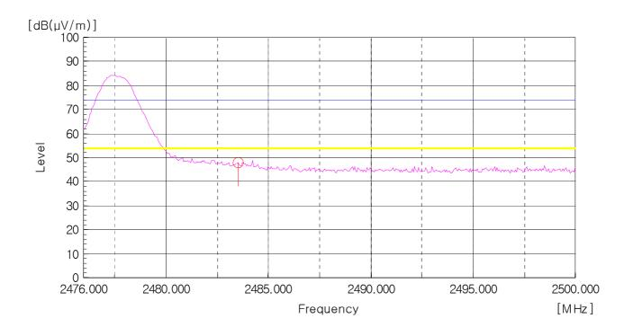
Peak Detector: RBW: 1MHz, VBW: 10Hz (2483.5 MHz - 2500 MHz), Worst case (121CH, Horizontal)
