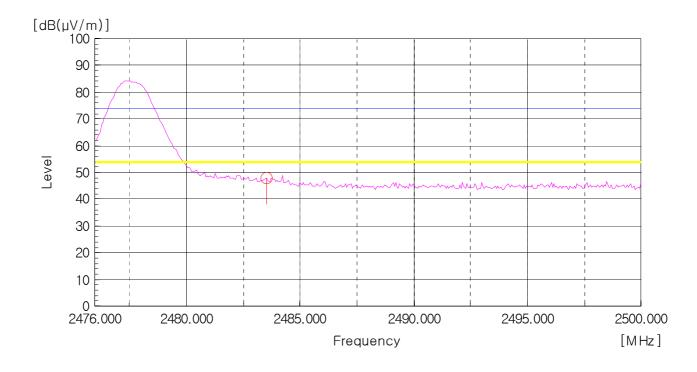
Peak Detector: RBW: 1MHz, VBW: 10Hz (2483.5 MHz - 2500 MHz), Worst case (121CH, Horizontal)
