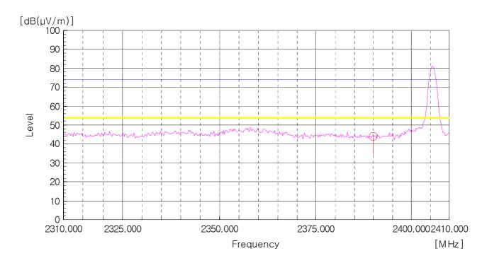
AV Detector: RBW: 1MHz, VBW: 10Hz (2310 MHz - 2390 MHz)
