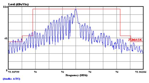
Top Plot is with a RES BW: 300 Hz and VIDEO BW: 300 Hz, but occupied bandwidth fails emission mask in Peak Mode.
