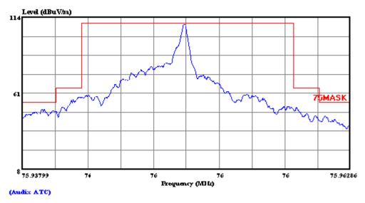
Top Plot is with a RES BW: 300Hz and VIDEO BW: 10Hz. Occupied Bandwidth passes the emission mask in Average Mode using a **linear VIDEO BW of 10Hz.**
