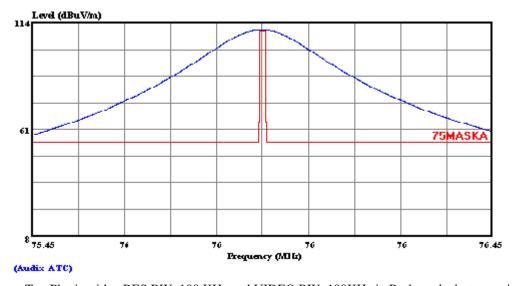
Top Plot is with a RES BW: 100 KHz and VIDEO BW: 100KHz in Peak mode, but occupied bandwidth fails emission mask due to a large RES BW setting.
