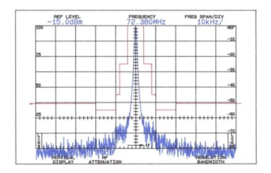
FCC ID: IFHFLA54SX OCCUPIED BANDWIDTH UNMODULATED CARRIER
