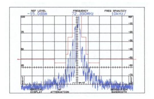
FCC ID: IFHFLA54SX OCCUPIED BANDWIDTH RBW 1 kHz, No Video Filter
