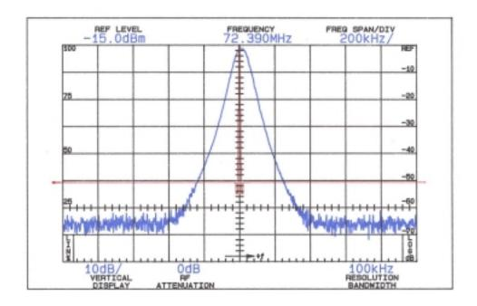
FCC ID: IFHFLA54SX OCCUPIED BANDWIDTH RBW 100 kHz, No Video Filtering
