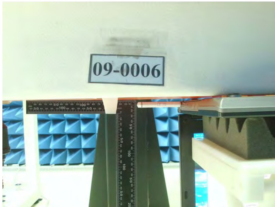
Figure 12. Body SAR Test Setup (Flat Section) _ EUT Horizontal Up_LCD Open 90°_5mm
