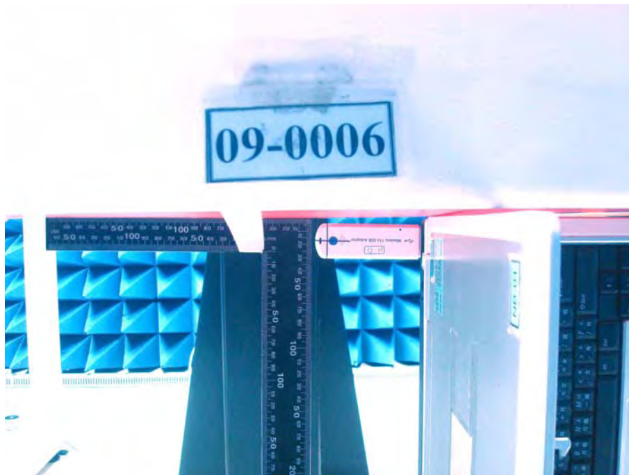
Figure 17. Body SAR Test Setup (Flat Section) _ Vertical Back_LCD Open 90°_5mm
