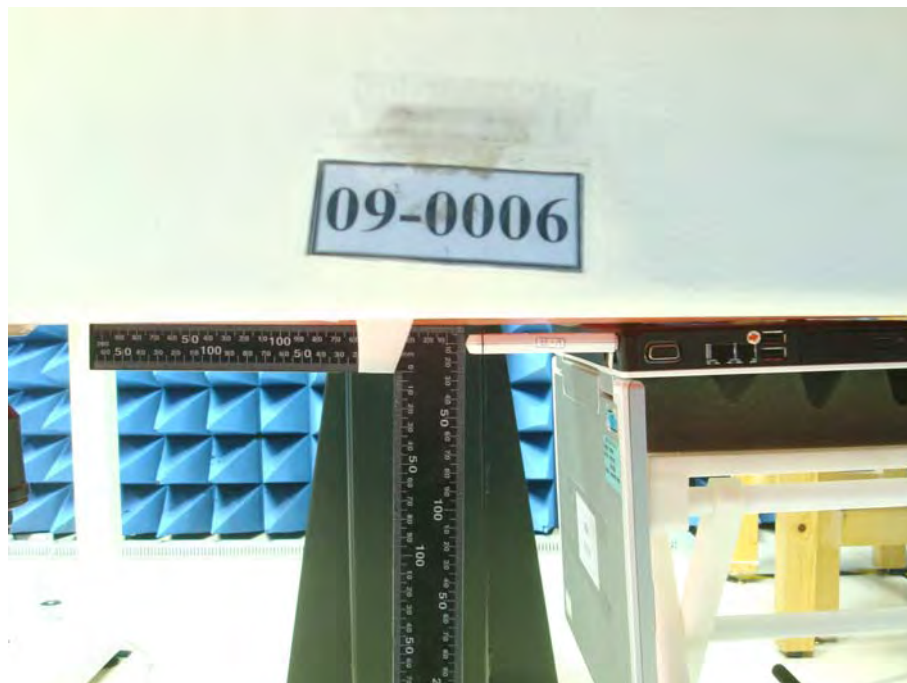
Figure 13. Body SAR Test Setup (Flat Section) _ EUT Horizontal Up_LCD Open 90°_5mm_ NB of Vertical
