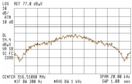
Note that the 20 dB points are referenced to the display line which was placed at the fundamental peak when measured with a 100 kHz bandwidth. The field strength was not maximized for this measurement. The 20 dB bandwidth falls within the central 80% of the band, demonstrating compliance to 15.215(c).
