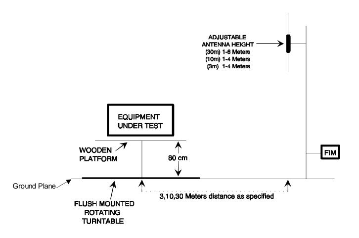
Radiated Test Setup and Procedure - cont'd
