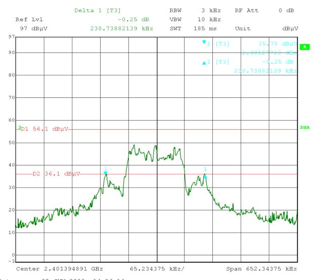
Date: 25.JUN.2009 14:36:14 V7E-VP 2.4 GHz transmitter 20 dB Bandwidth, 230.7 kHz
