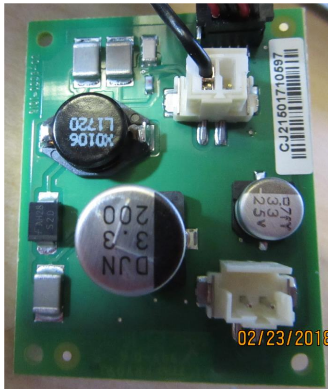
IDI-VLU10 Regulator PCB Top Side
