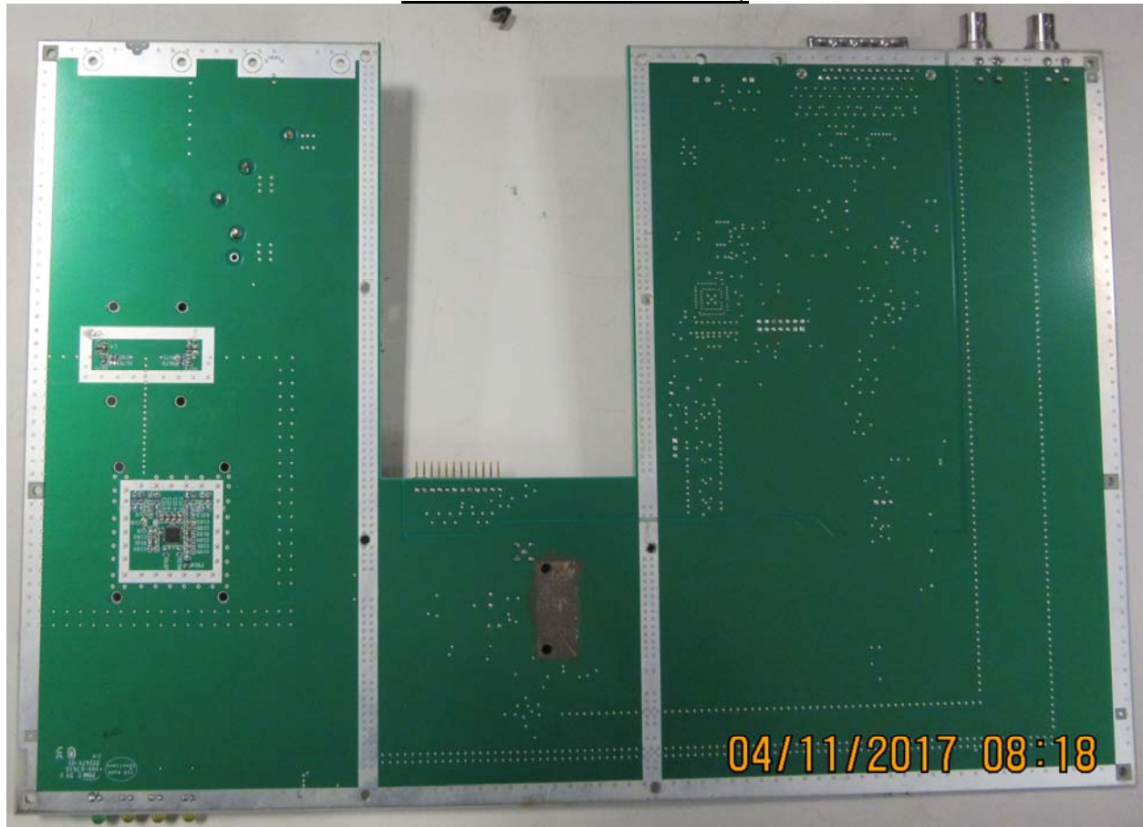
Figure 3PA600 T/R Switch and control PCB Bottom
