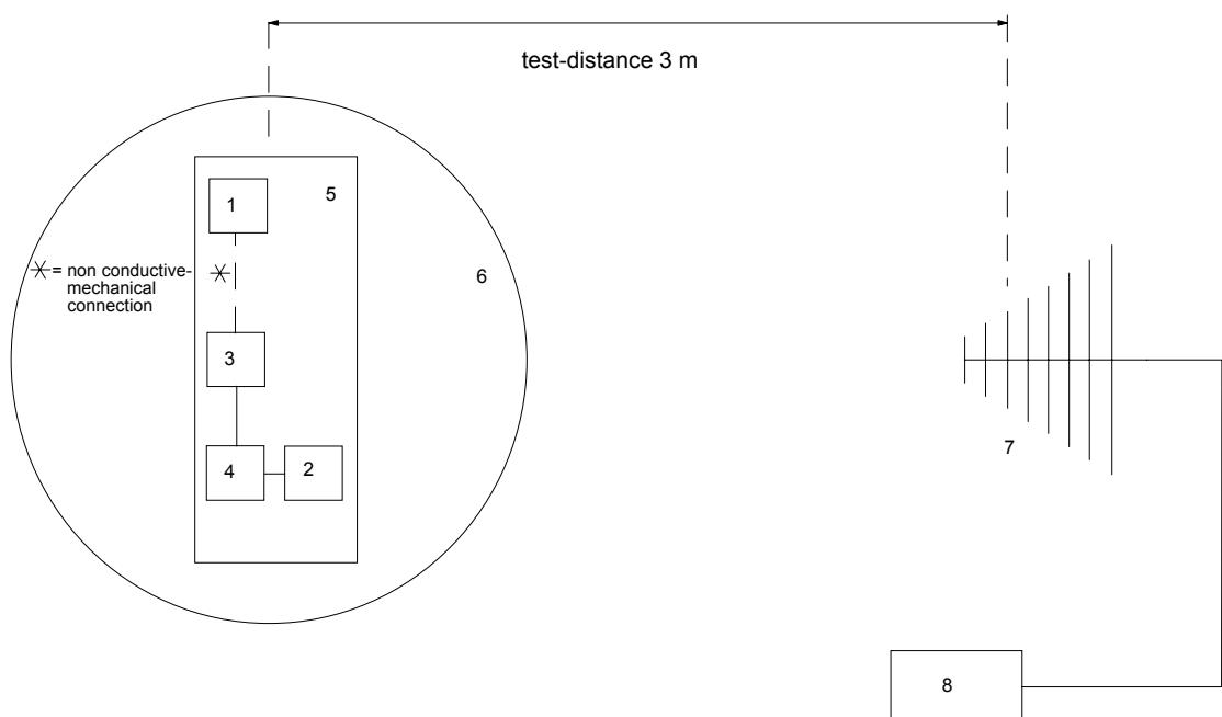
Figure 1: Measurement setup for radiated emission test
