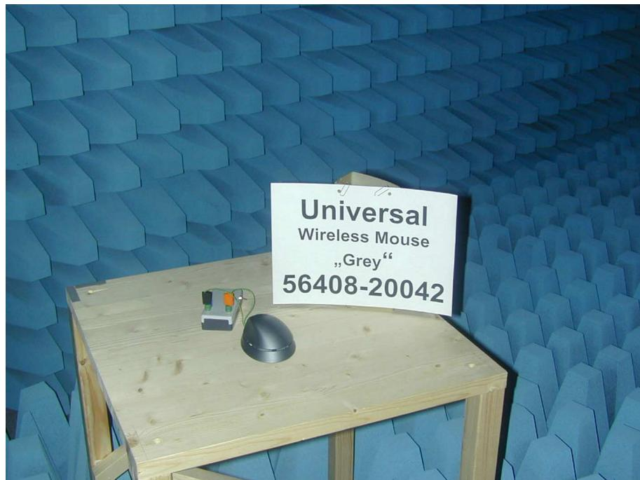
**7.2. Radiated Emissions 30 – 1000 MHz (Final Test in Open Area Test-Site)**
