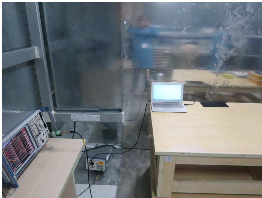
FCC RADIATED EMISSION TEST SETUP
