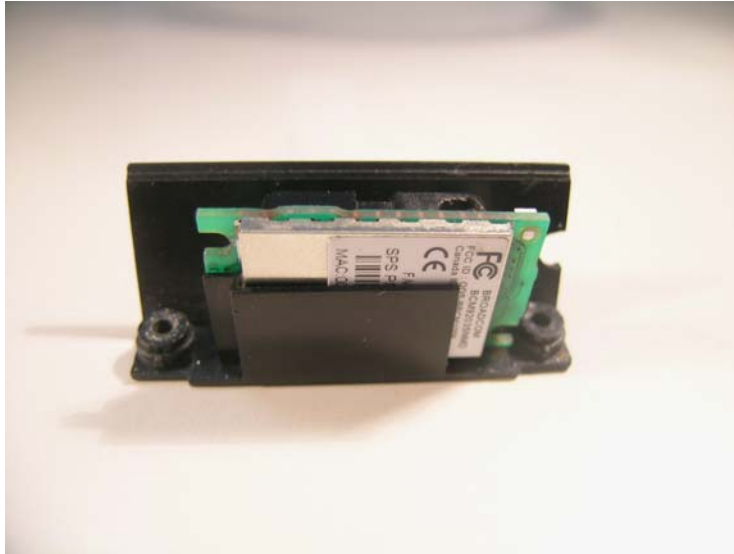
Antenna Module mounted in plastic Holder
