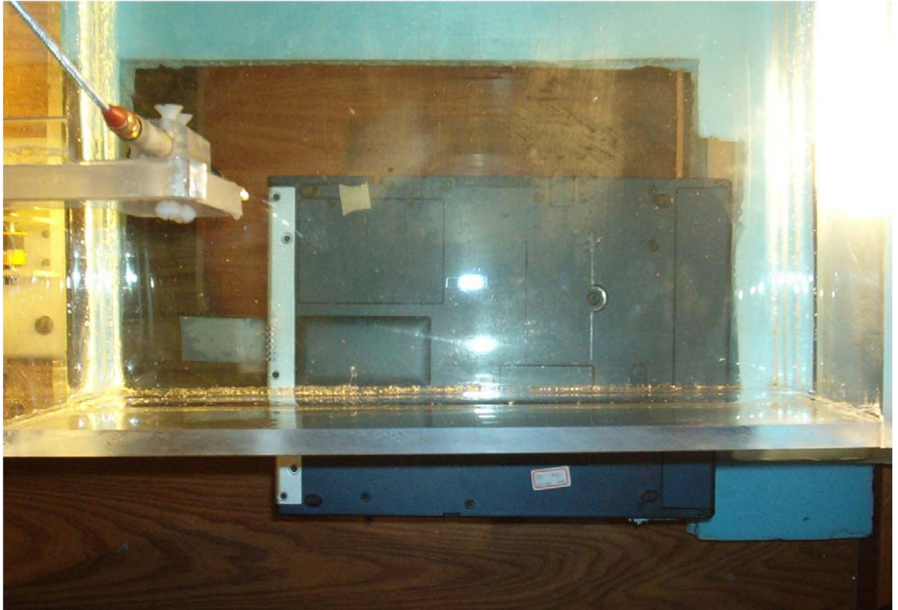
a. Wireless LAN antenna parallel to the Tablet.
