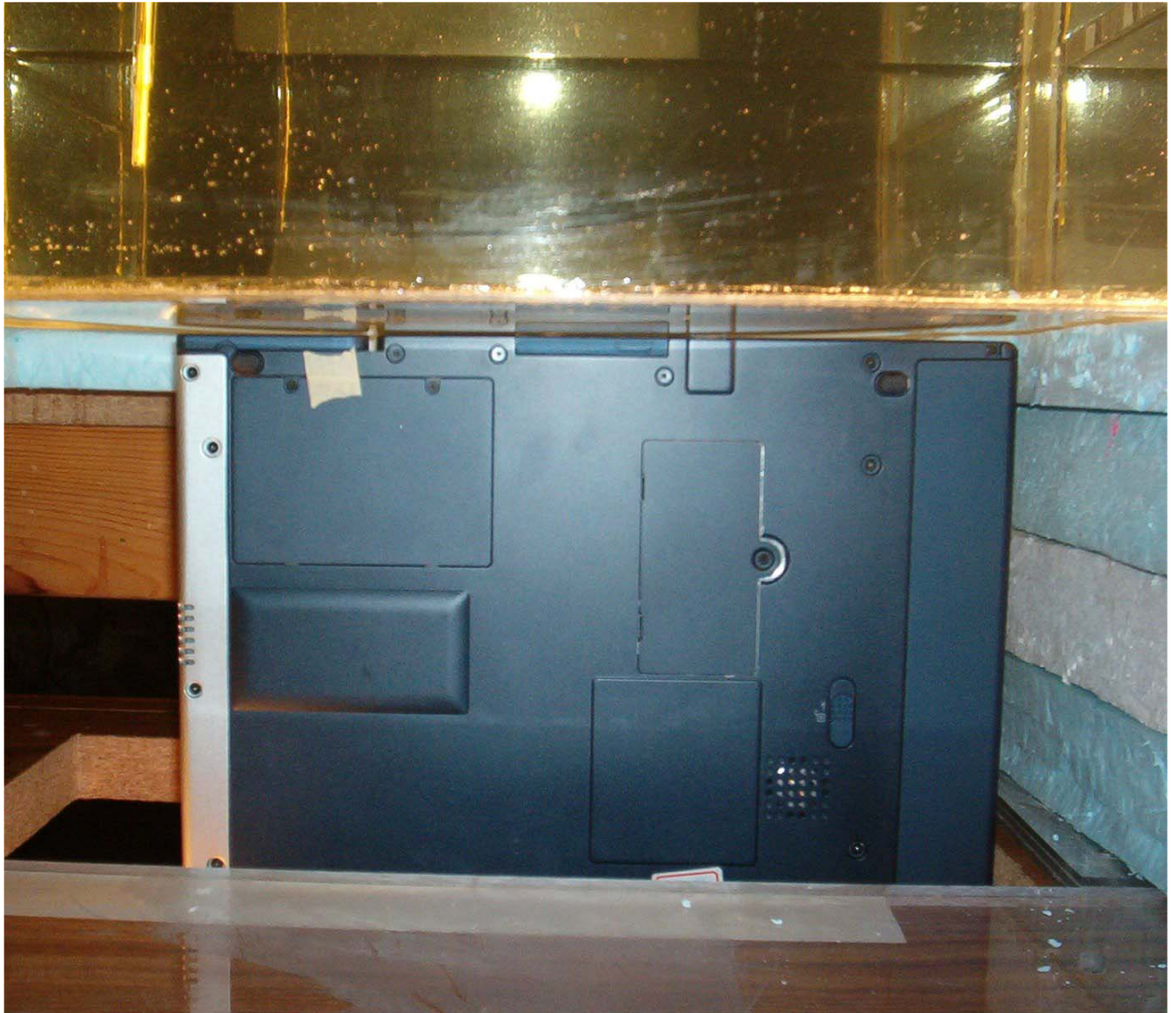
a. Wireless LAN antenna parallel to the Tablet.
