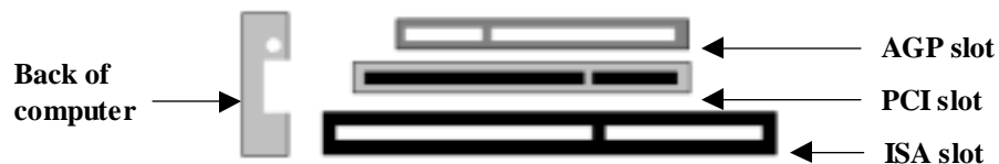
AGP vs. PCI vs. ISA expansion slots
