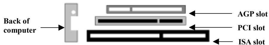
AGP vs. PCI vs. ISA expansion slots
