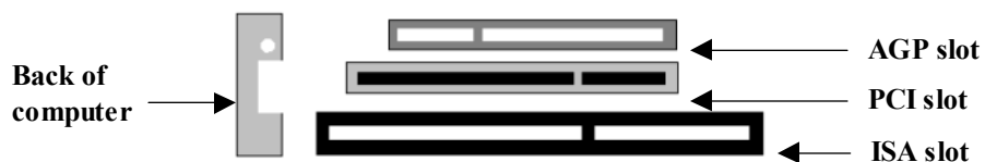
AGP vs. PCI vs. ISA expansion slots
