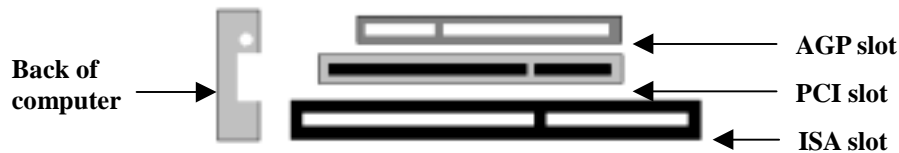
AGP vs. PCI vs. ISA expansion slots
