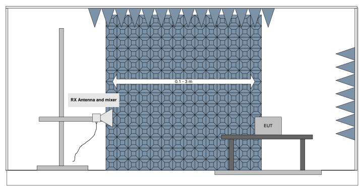
Note: The antenna is actually manipulated by hand as per the TCB Council Millimeter Wave Test Procedure document.
