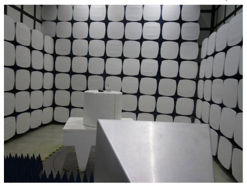
1.2 Radiated Spurious Emissions Test Setup
