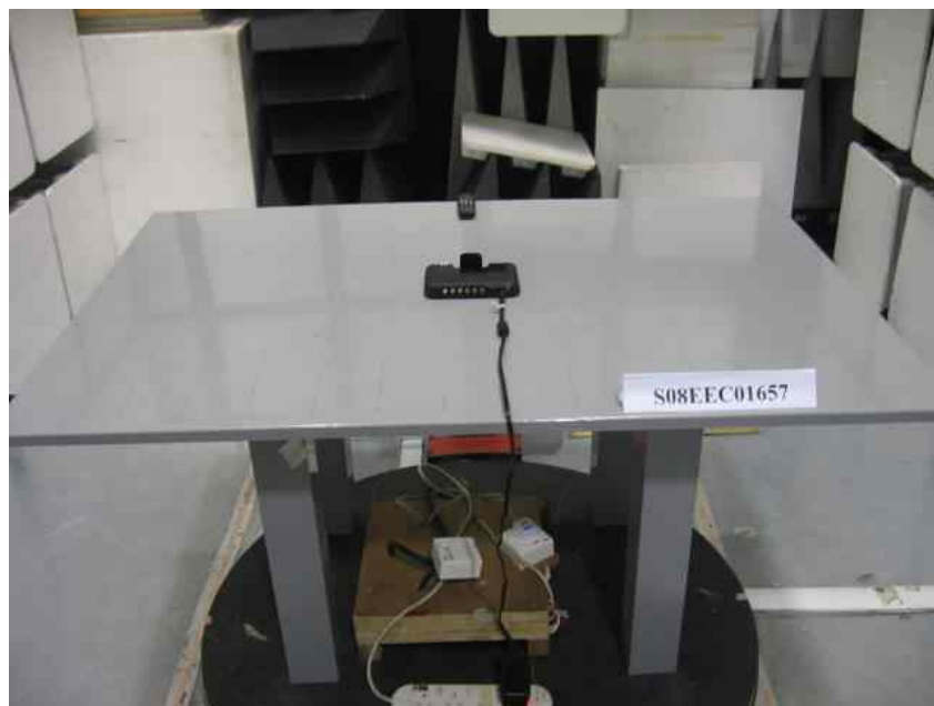
Radiated Emissions Test Setup (Rear View)
