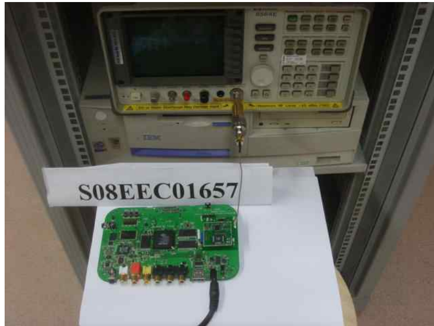
Spectrum Bandwidth (6dB Bandwidth Measurement) Test Setup
