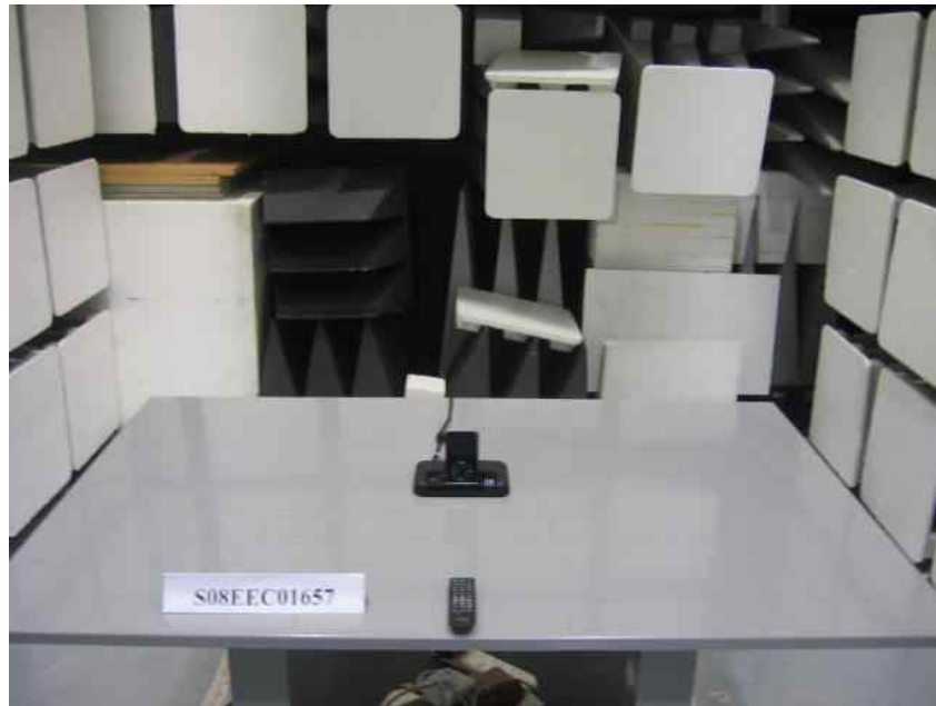
Band Edge Compliance (Radiated) Test Setup
