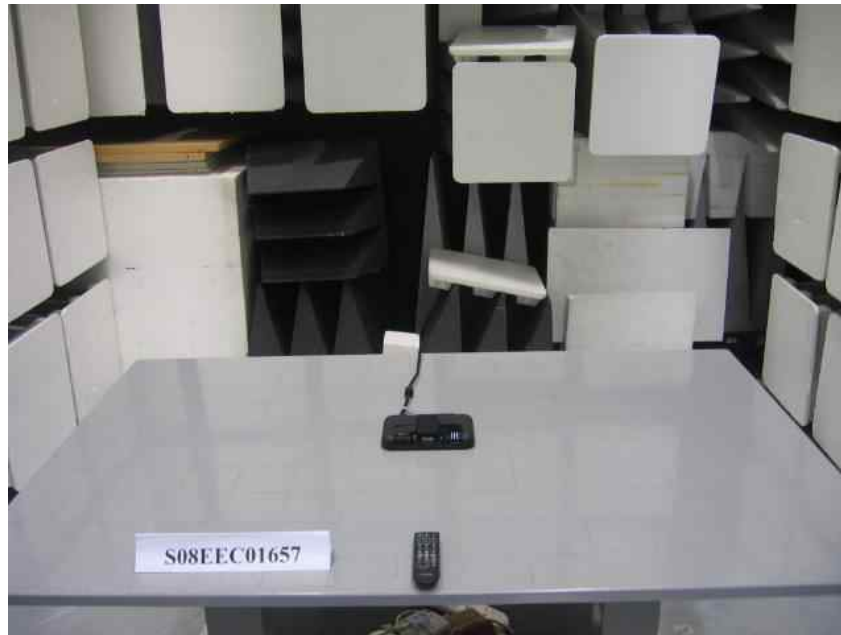
Radiated Emissions Test Setup (Front View)
