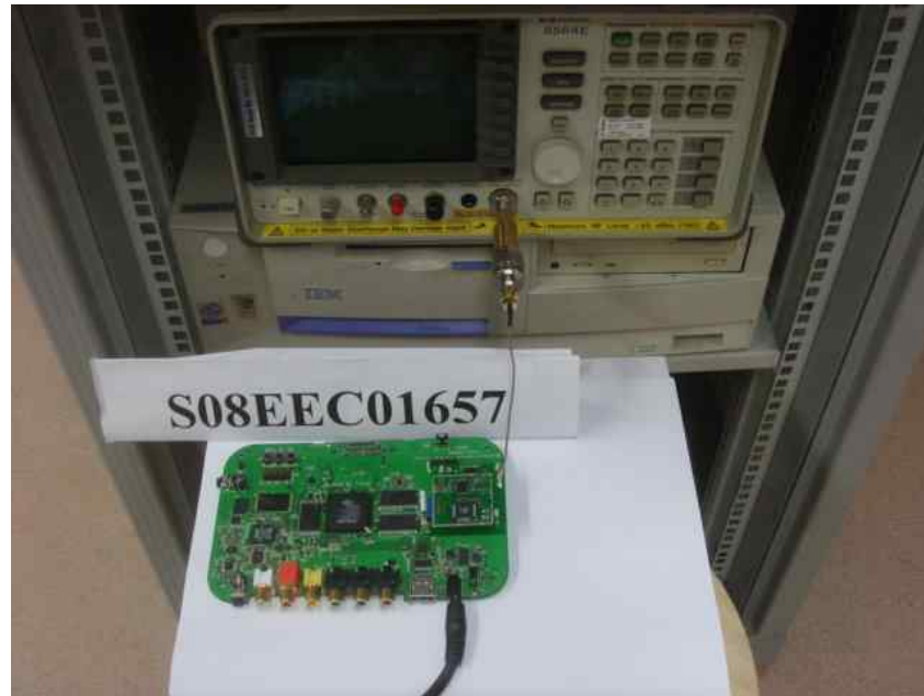
Band Edge Compliance (Conducted) Test Setup
