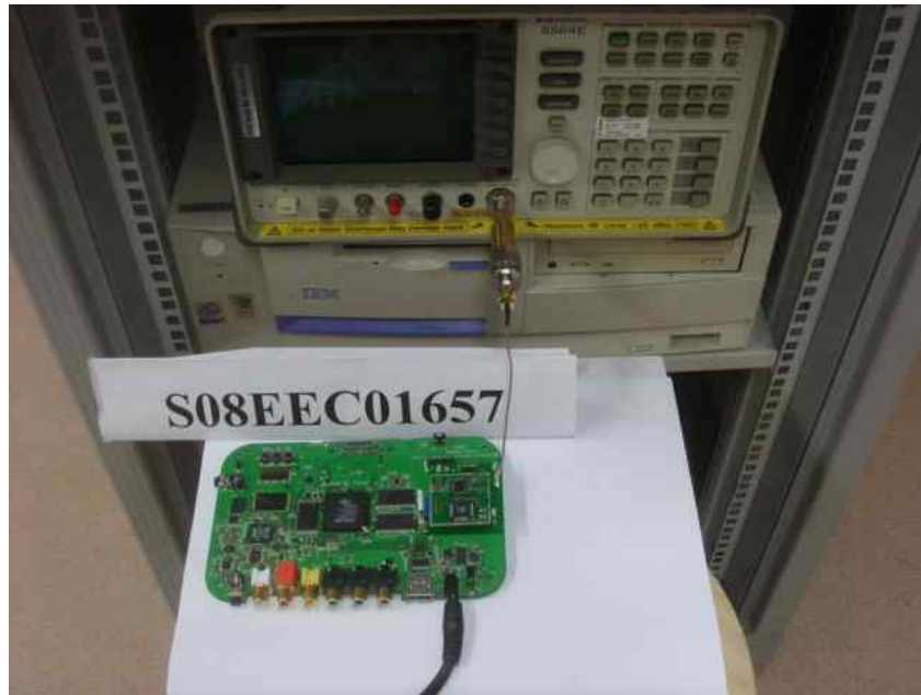
Peak Power Spectral Density Test Setup
