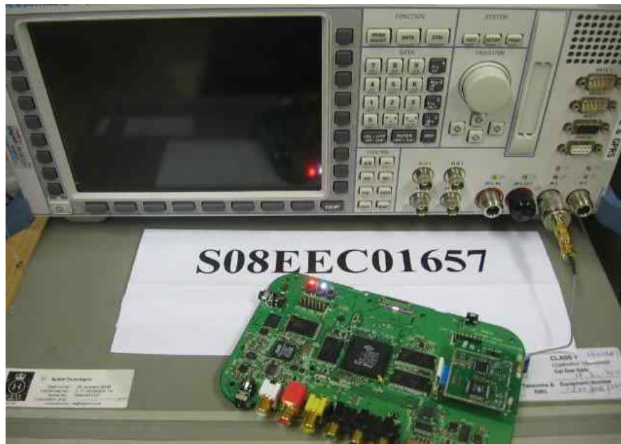
Maximum Peak Power Test Setup
