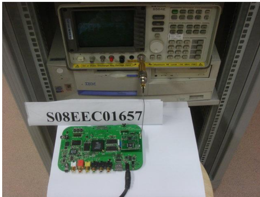
RF Conducted Spurious Emissions Test Setup
