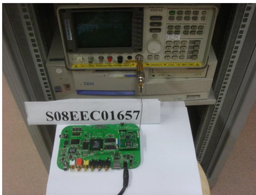
Band Edge Compliance Test Setup
