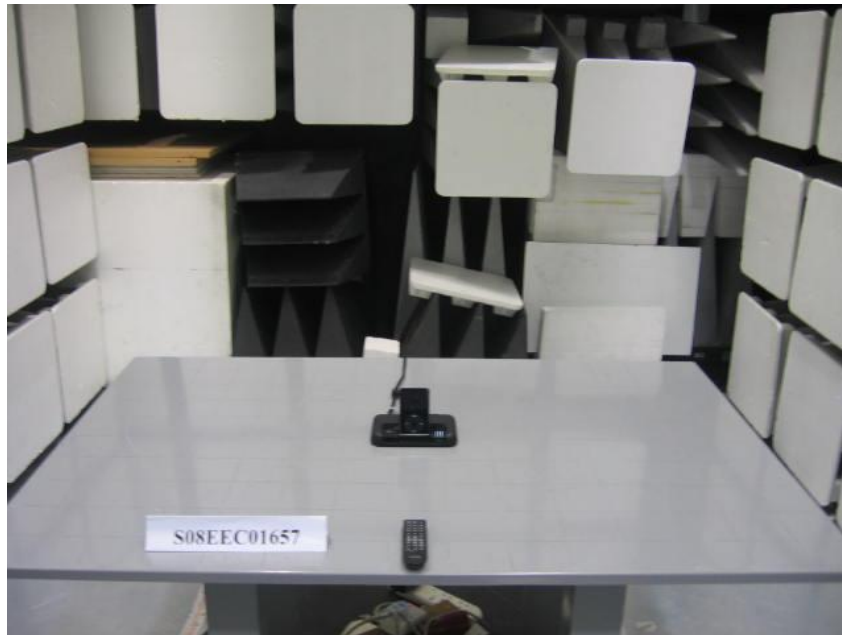
Band Edge Compliance (Radiated) Test Setup
