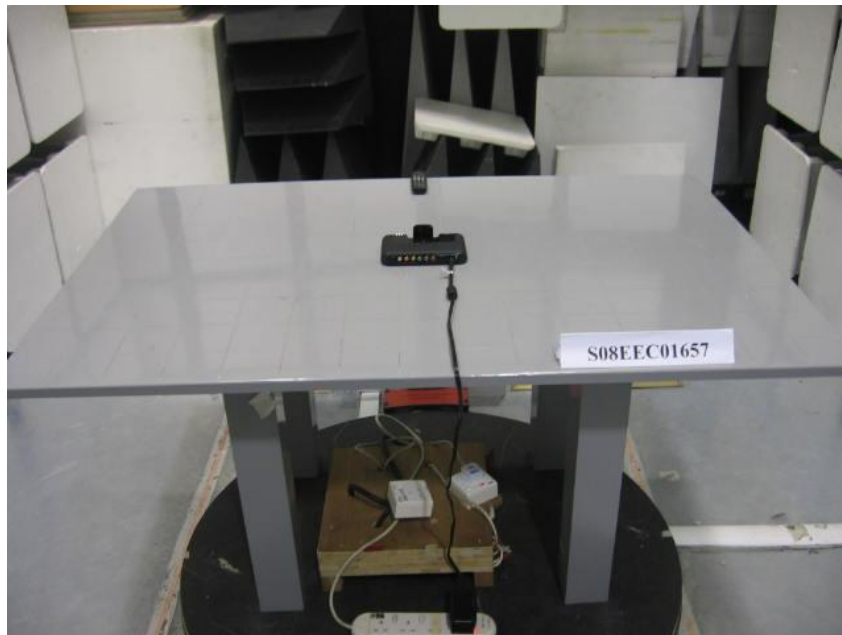
Radiated Emissions Test Setup (Rear View)
