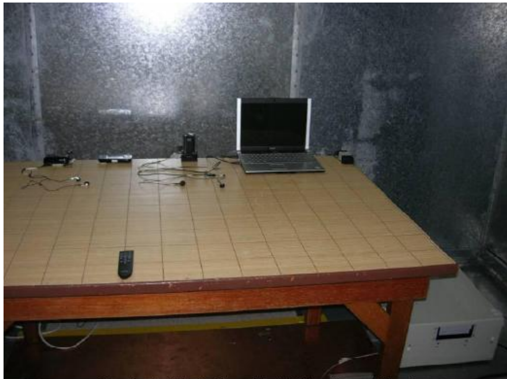
Conducted Emissions Test Setup (Front View)
