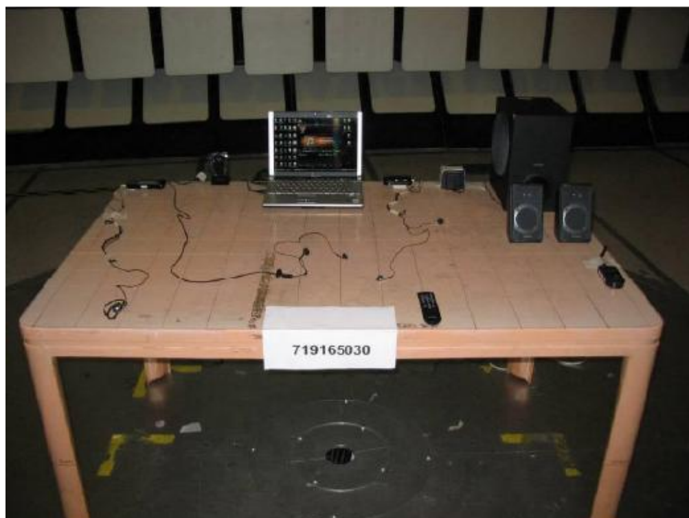
Radiated Emissions Test Setup (Front View)
