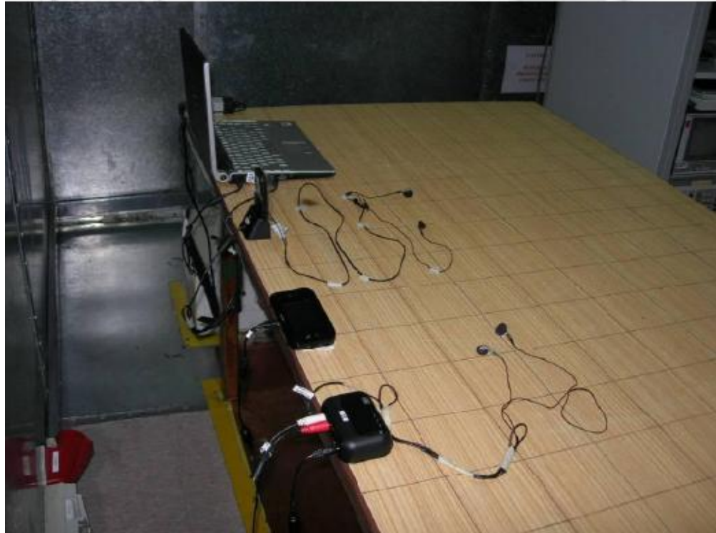
Conducted Emissions Test Setup (Rear View)
