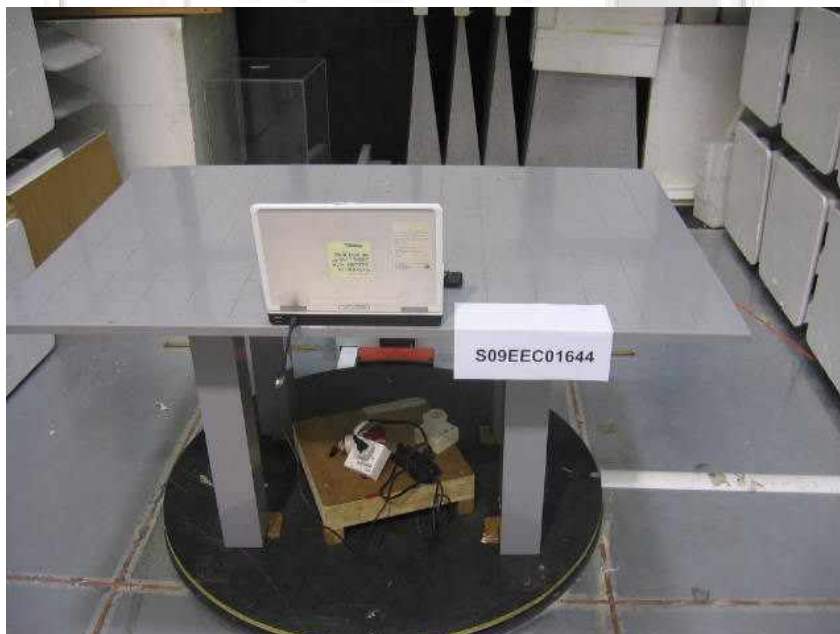
Radiated Emissions Test Setup (Rear View)
