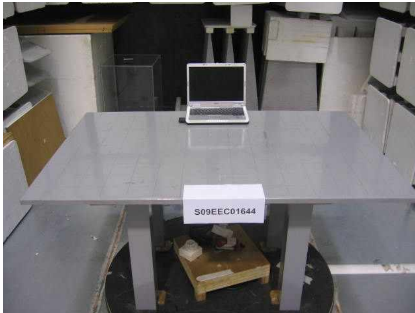
Radiated Emissions Test Setup (Front View)
