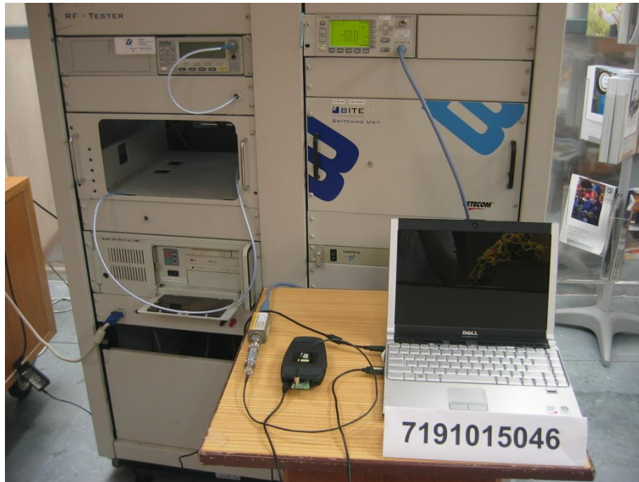
Maximum Peak Power Test Setup
