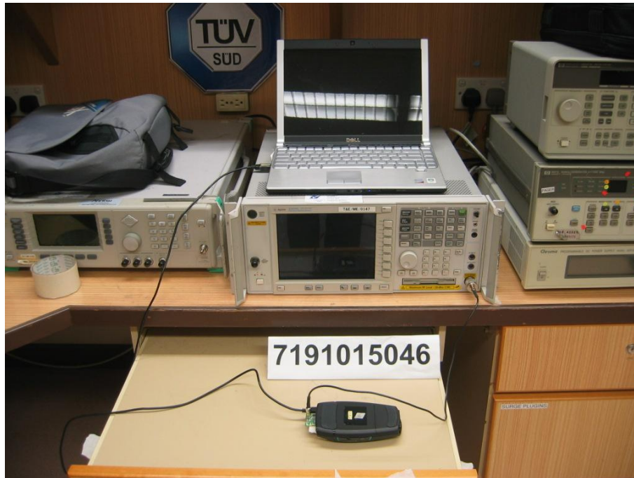
Peak Power Spectral Density Test Setup
