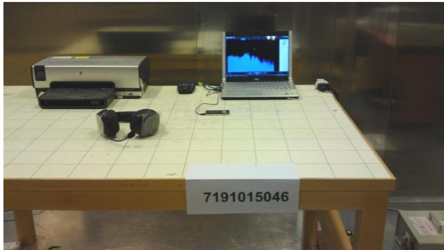
Conducted Emissions Test Setup (Front View)
