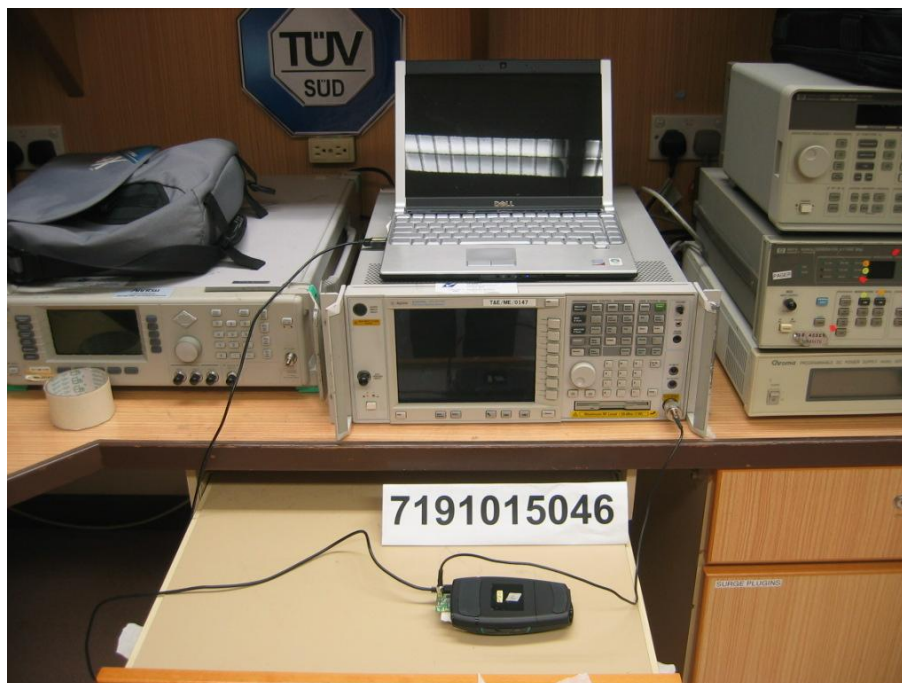
Spectrum Bandwidth (6dB Bandwidth Measurement) Test Setup
