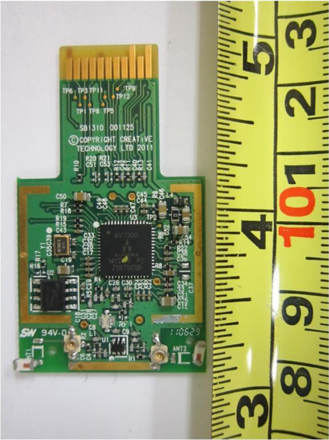
RF Module Circuit with RF Shield Removed Component View
