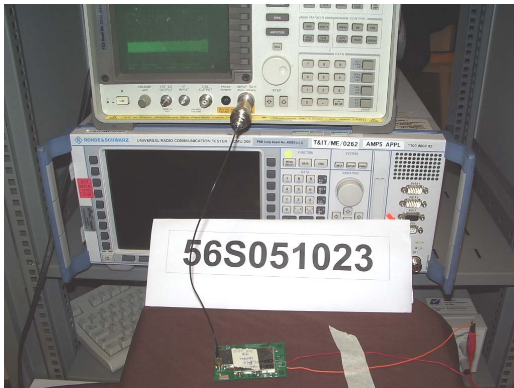
Peak Power Spectral Density Test Setup MAXIMUM PERMISSIBLE EXPOSURE (MPE) TEST
