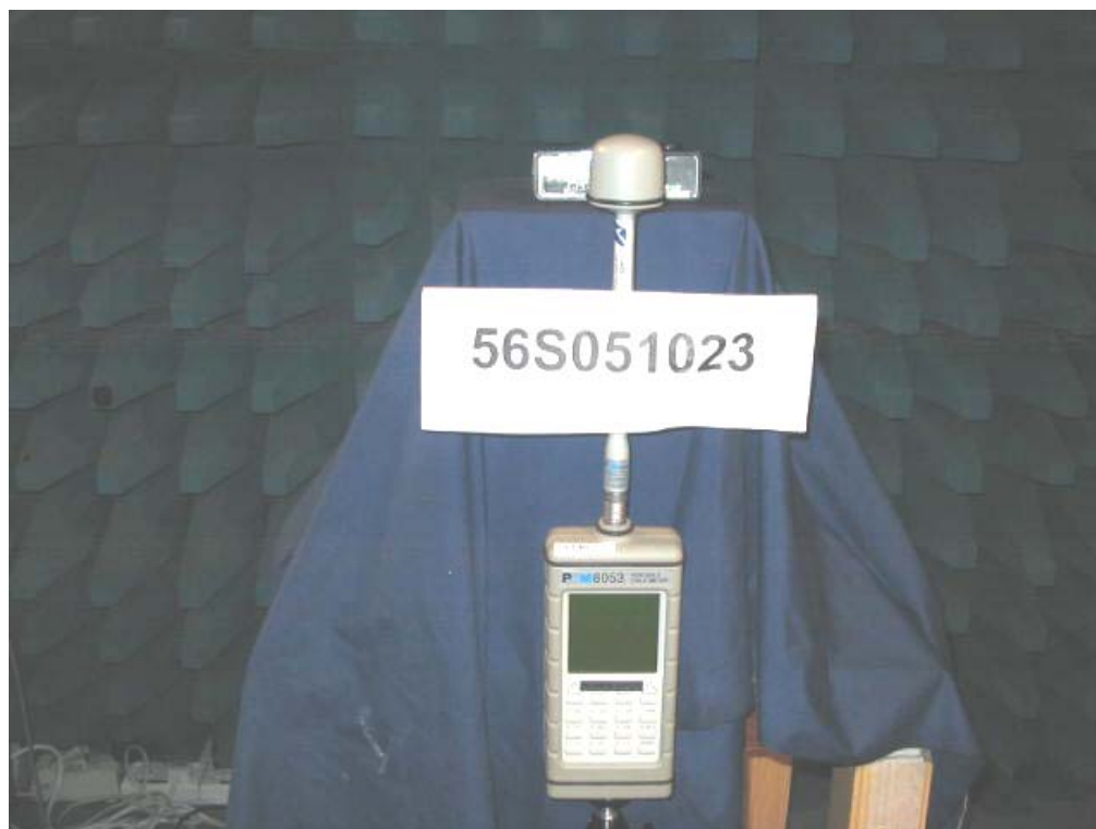
Maximum Permissible Exposure (MPE) Test Setup
