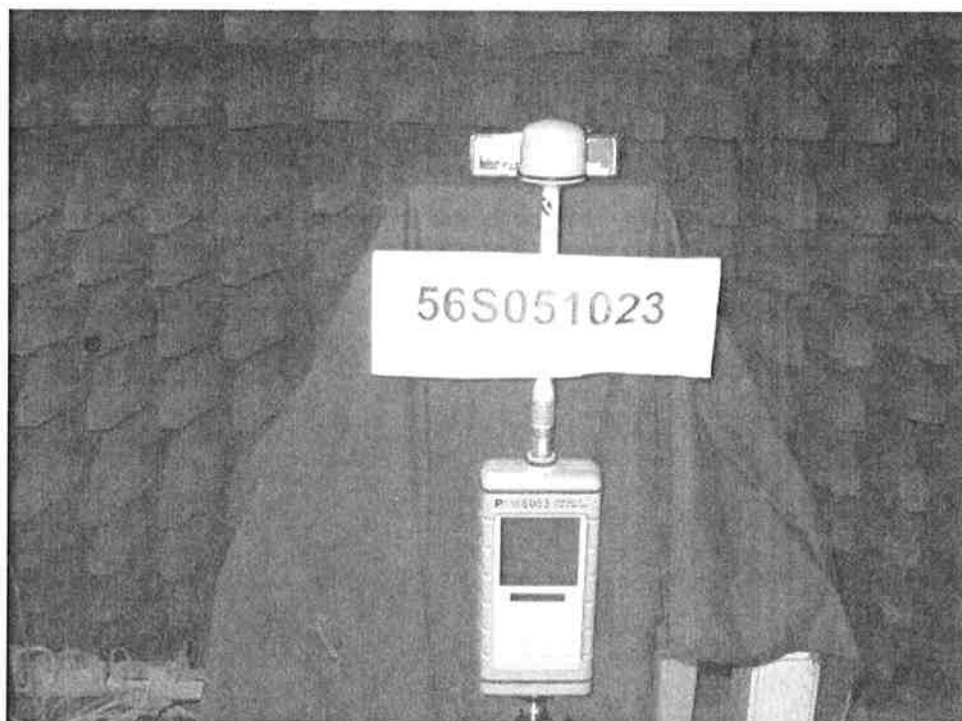
Maximum Permissible Exposure (MPE) Test Setup
