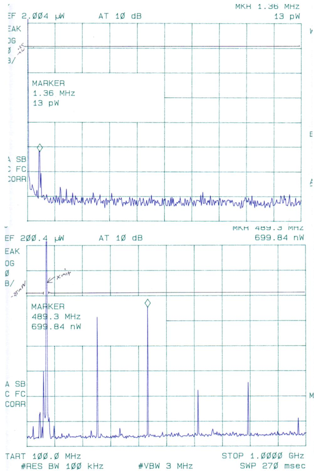
**VIII. Measurement Results for AIS Physical Tests Cont'd:****12. Conducted Spurious.**
