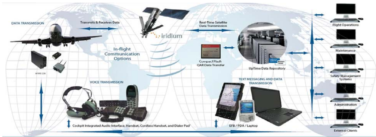
Figure 2-1 – Airbus Iridium SATCOM System Operational Concept
