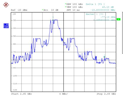
At the upper bandedge, the attenuation is about 48.1 dB. Field strength at the bandedge = 81.5 – 48.1 = 33.4 dBuV/m at 3m which is less than the general limit of 54.0 dBuV/m
