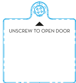
BE-226 Battery door engraving Emboss 0.3mm
