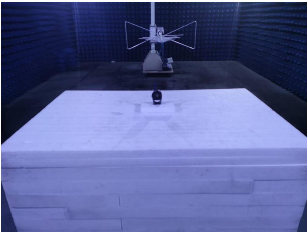
Photo of Radiated Emission Measurement (Below 1G)
