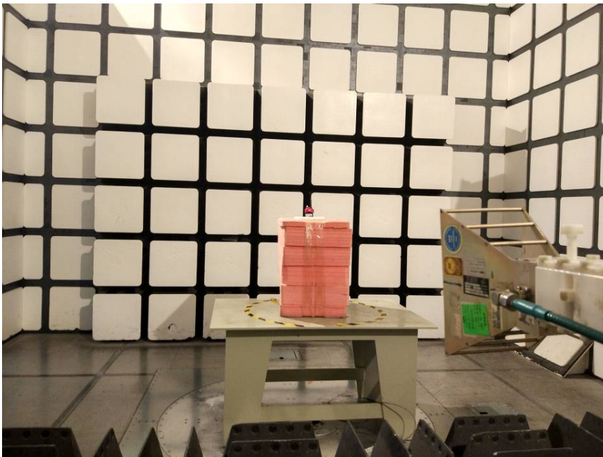
Radiated Emissions View (Above 1 GHz)
