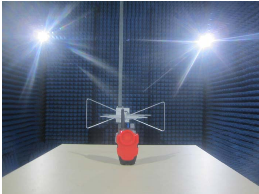
Radiation Emission Test Setup (30MHz to 1GHz)
