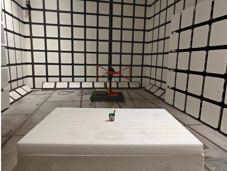
Radiated Emissions View (Below 1 GHz)
