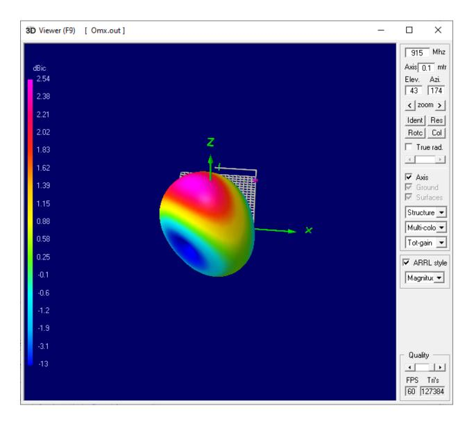
Max Gain= 2.54dBi. (Average Gain Test error result=+/-0.3dB)
