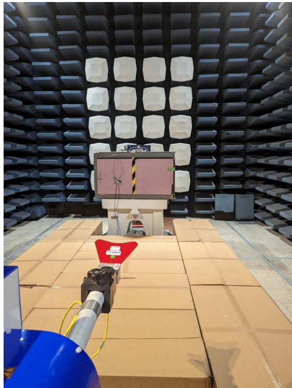
Figure 55: Radiated Emissions Setup: 1 GHz - 18 GHz
