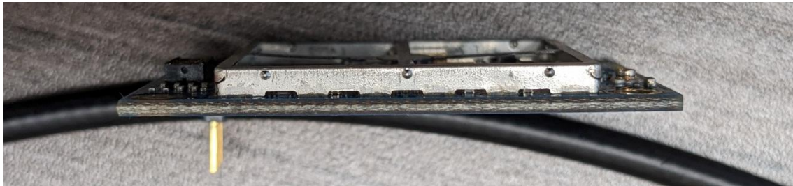
Figure 3 XPD2400 board's side view with shield lid removed.
