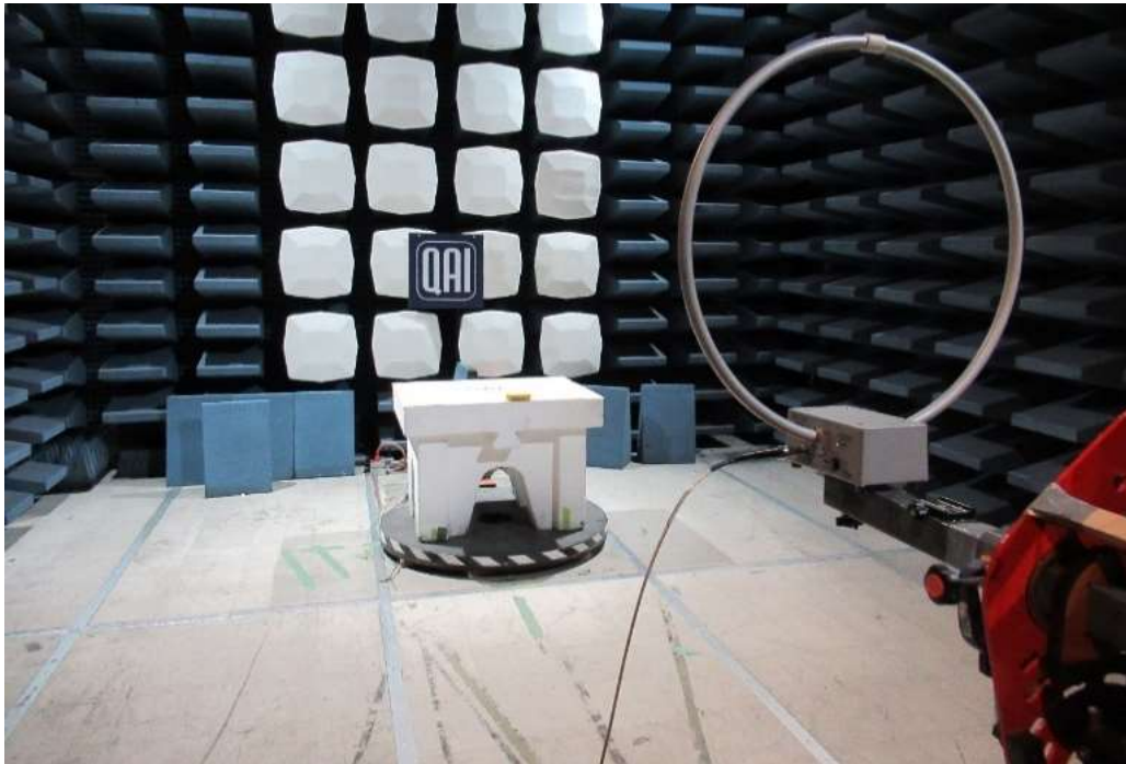
Figure 1: Radiated Emissions performed at the 3m SAC, 150kHz – 30MHz
