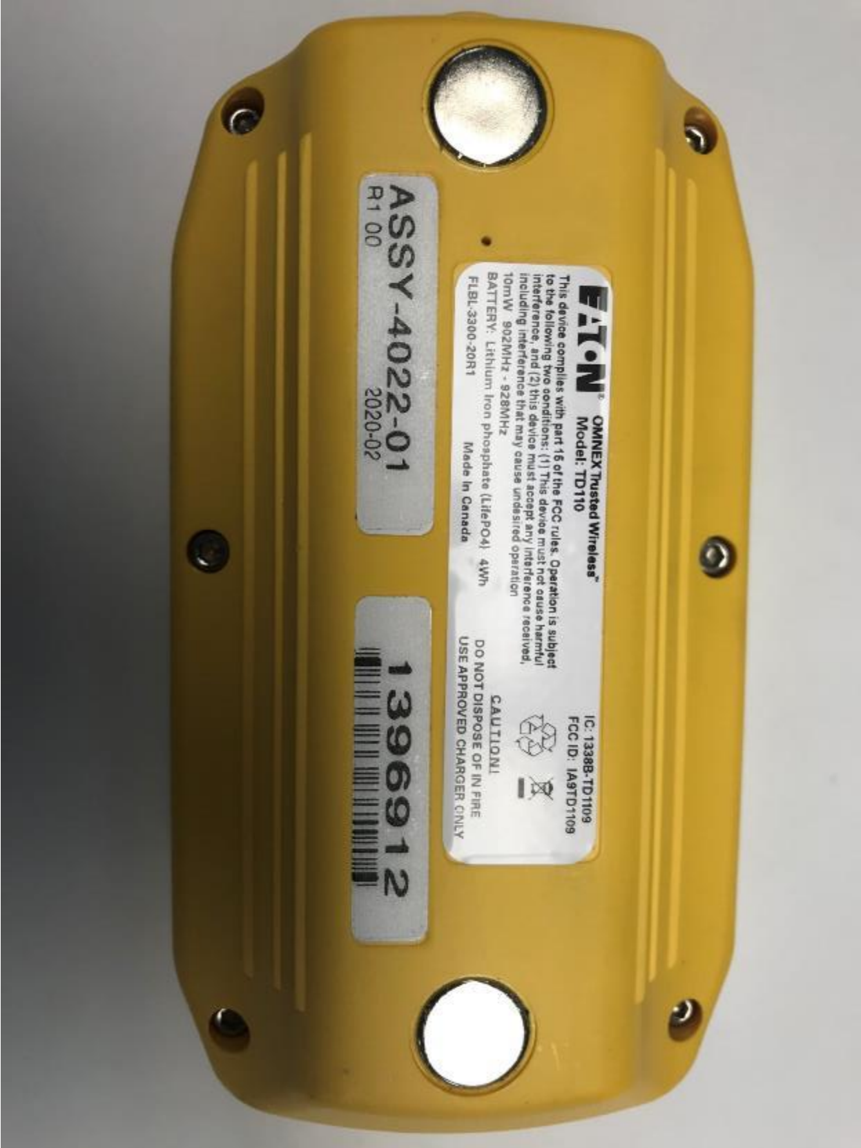
FCC/IC Label Location: TD110 Back Side
