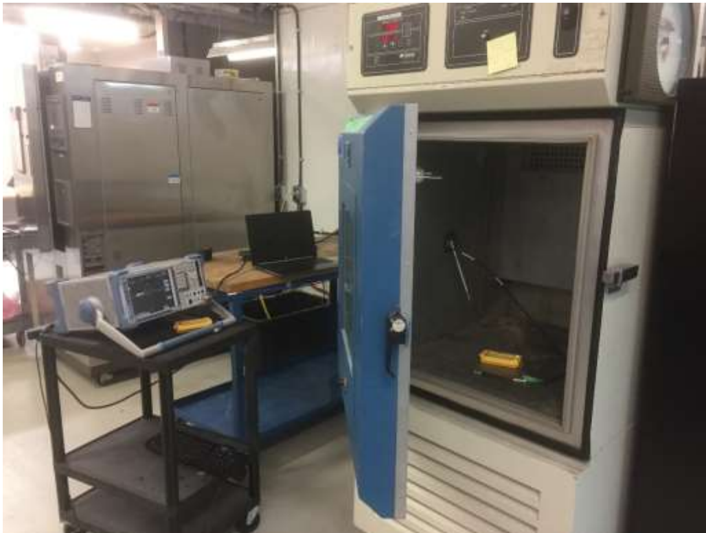
Figure 7: Frequency Stability Testing
