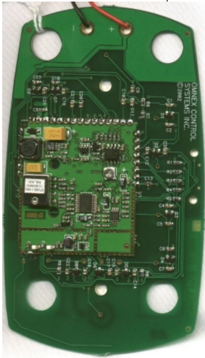
Module installed on Processor board: Component Side
