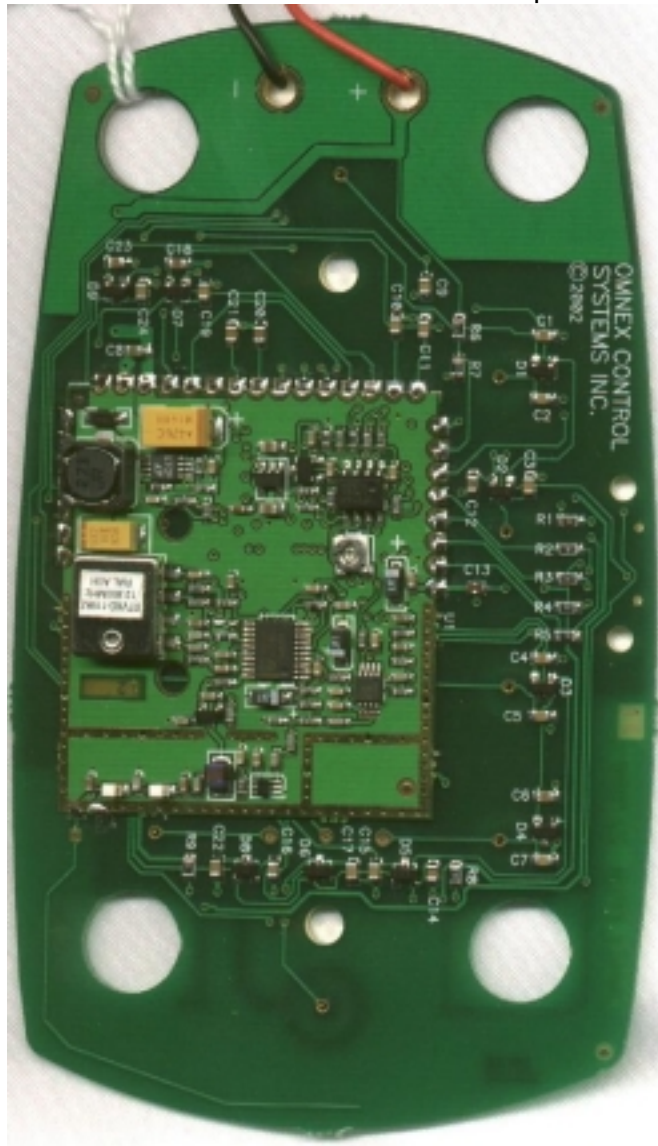
Module installed on Processor board: Component Side
